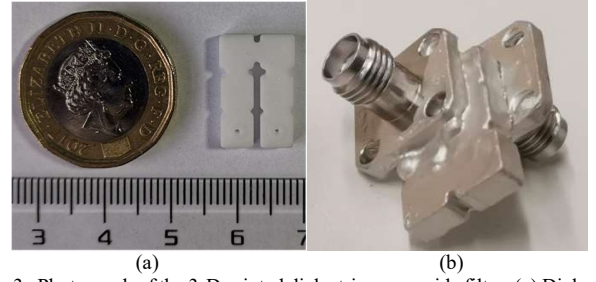
Fig. 3. Photograph of the 3-D printed dielectric waveguide filter: (a) Dielectric block after sintering; (b) Dielectric waveguide filter after silver plating with assembled SMA connectors.
