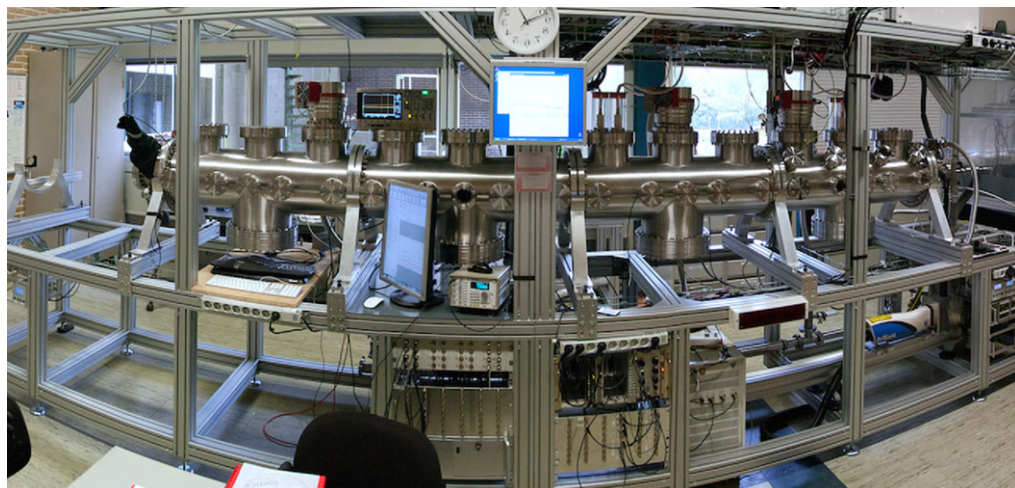
Figure 4. 4.5 m length Stark decelerator at Groningen designed to produce slow beams of heavy diatomic molecules for studying fundamental symmetry violations. Adapted from [114].
