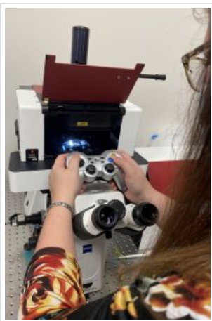
The optical trap pairs a laser with a microscope, enabling the laser beam to act like a pair of tweezers, with the ability to catch or ‘trap’ microscopic objects and move them around for study. Submitted photo
