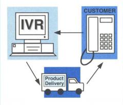
IVR software should not be confused with voice recognition software. The IVR system will not typically react to voice commands from the caller. However, IVR software is capable of integrating with voice recognition technology to increase its capabilities.
