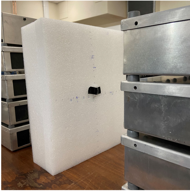
FIGURE 2. The spatial resolution tests are conducted using a 1 mm diameter resin bead placed inside a plastic sample holder and taped to a piece of polystyrene foam.
