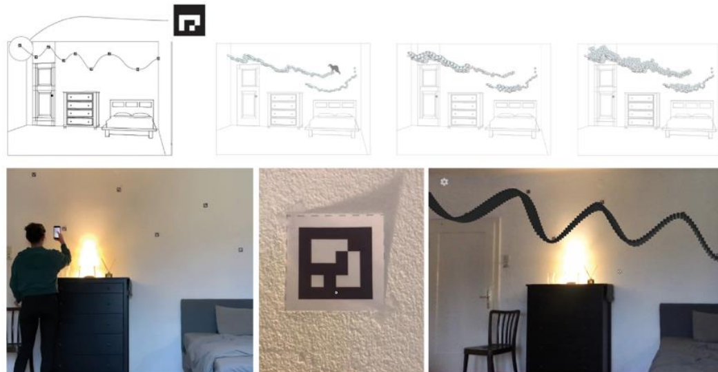
Fig.7: Project 1.1: “flow follows fologram”; design ideas (top), the process of scanning ArUco markers on the wall with the smartphone app, and adapting parameters with sliders in the ARapp, which are synchronized to the computer (Grasshopper window and Rhinoceros model window) (middle and bottom).98|eCAADe 39- CAAD and education - Volume 2
