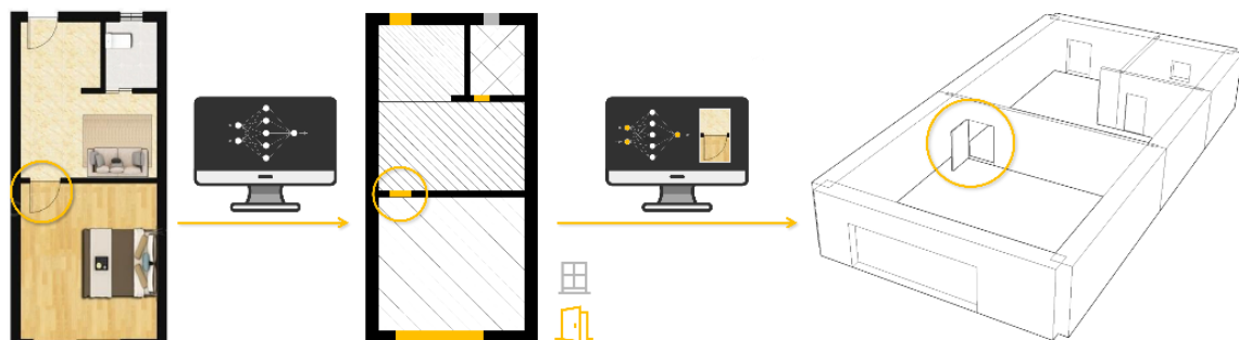
Fig.8: General process for door classification. The doors are recognized during segmentation, but the semantics are lost. We extract the zone where the door might be and use a classifier to recover that information. Floor plan image adapted from Lv et al.'s (2021) work.
