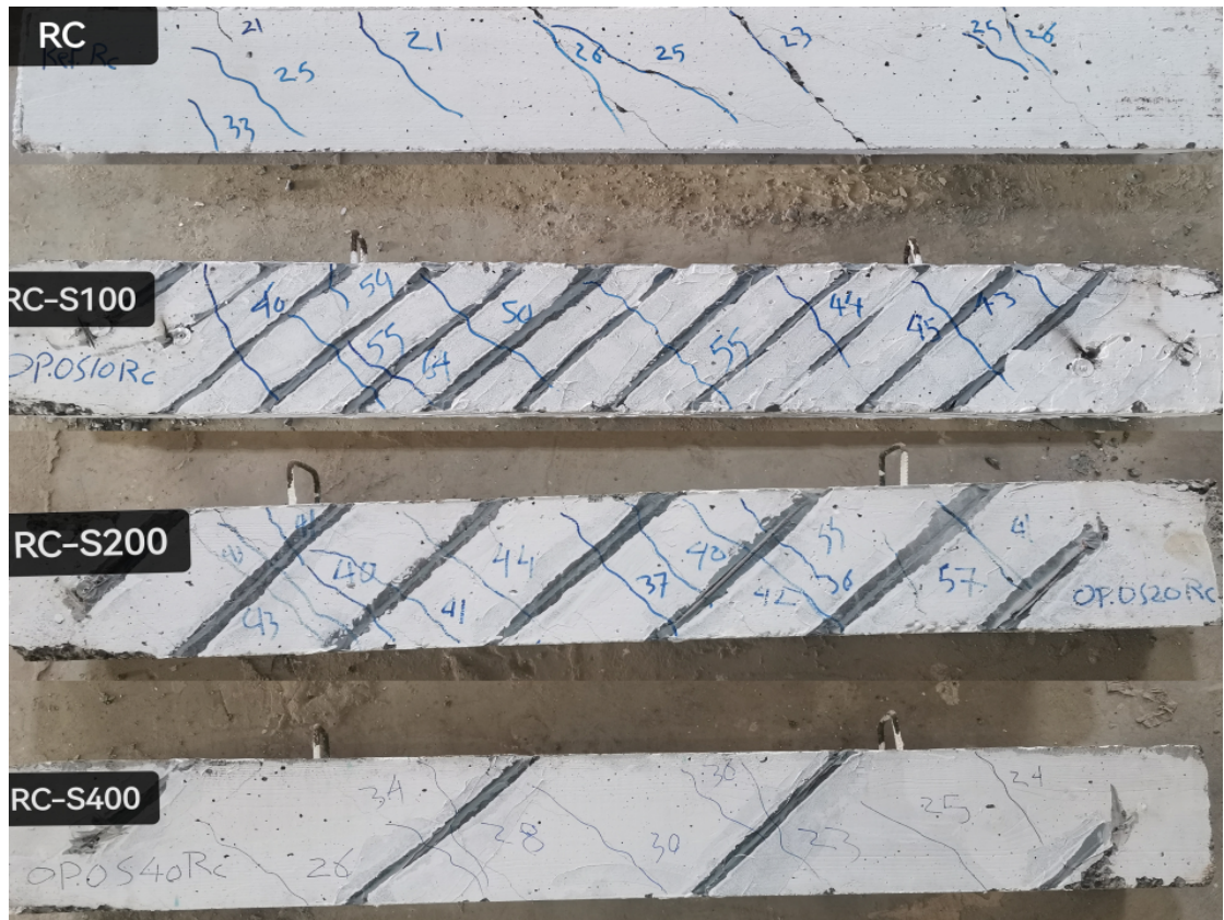
Fig. 15: Failure Mode for Beams under constant repeated load
