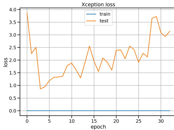
Fig. 7: Xception model transfer learning loss over 33 epochs of learning, learning rate=0.0001 and a batch of size 8 images per iteration.
