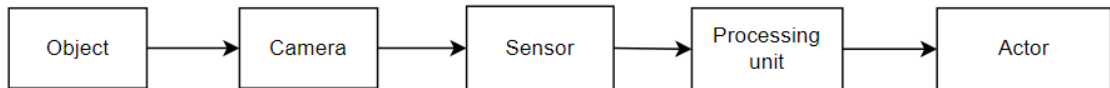
Figure 1. Chain of steps in a basic vision system. Based on source [4 p.3].
