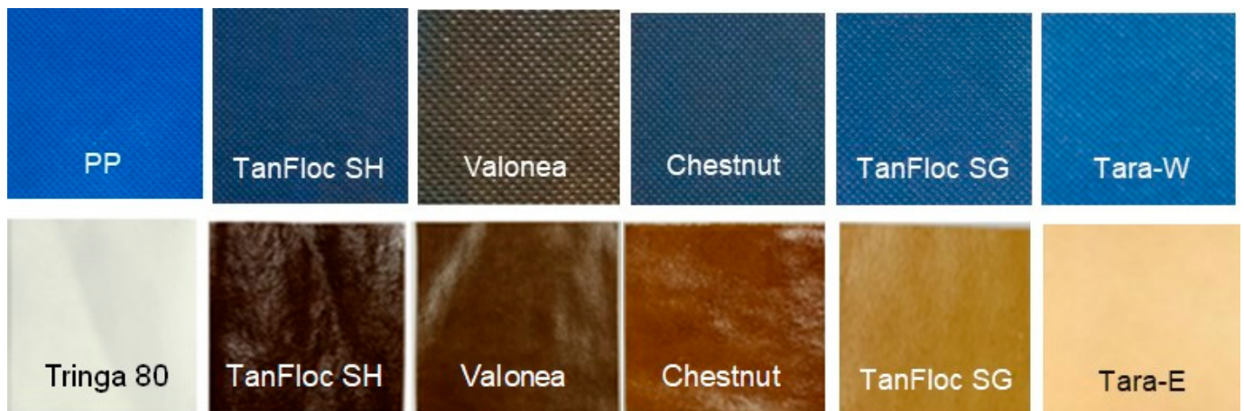
Figure 4. Uncoated and tannin-coated PP (top row) and Tringa 80 viscose (bottom row) privacy curtains.
