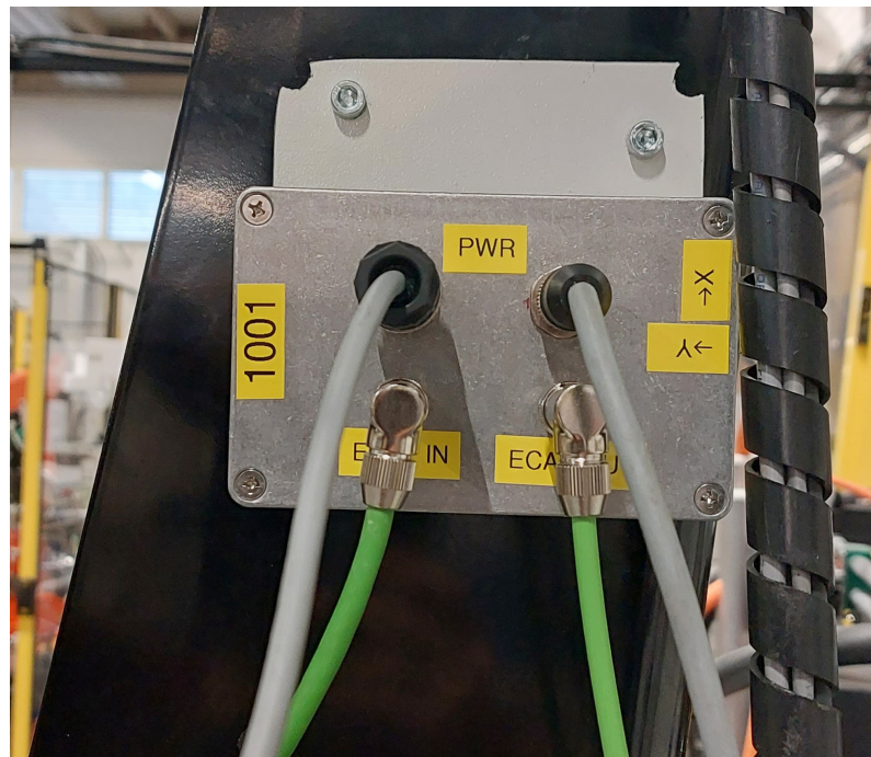
Figure 3.5. A completed sensor node, installed onto the Hiab hydraulic boom.
