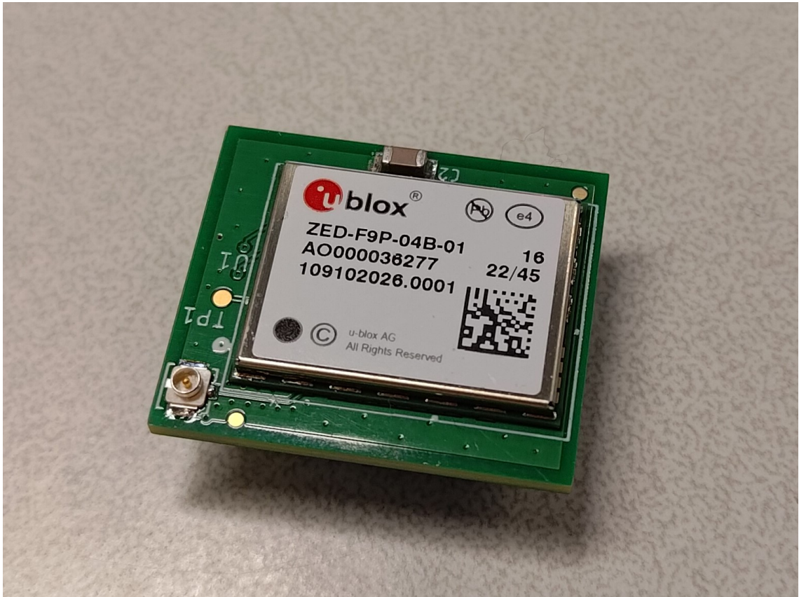
Figure 2.10. A u-blox ZED-F9P GNSS RTK chip mounted on a custom sensor module board with supporting components.
