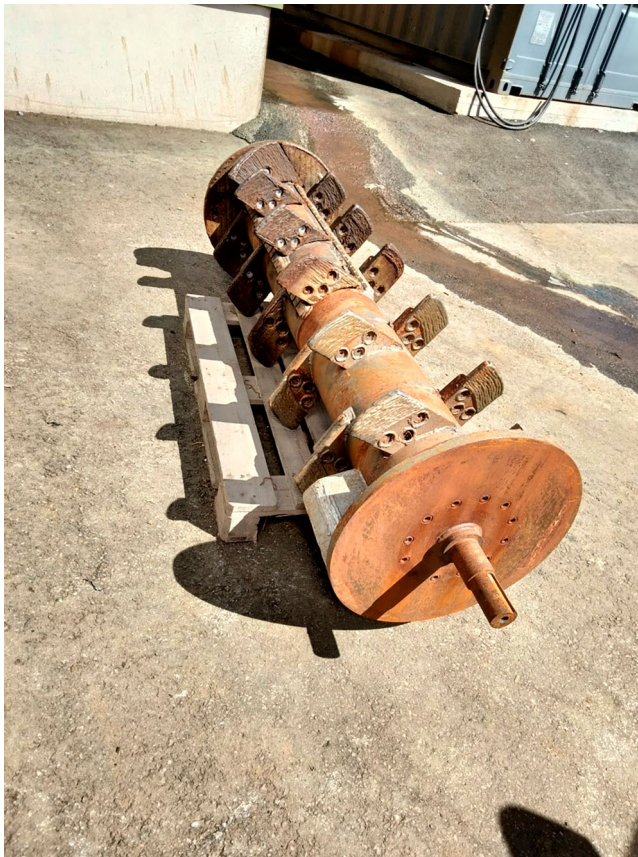
Figure 2. A worn 'screw' used in biowaste pretreatment machinery to separate plastic and metal from biowaste.
