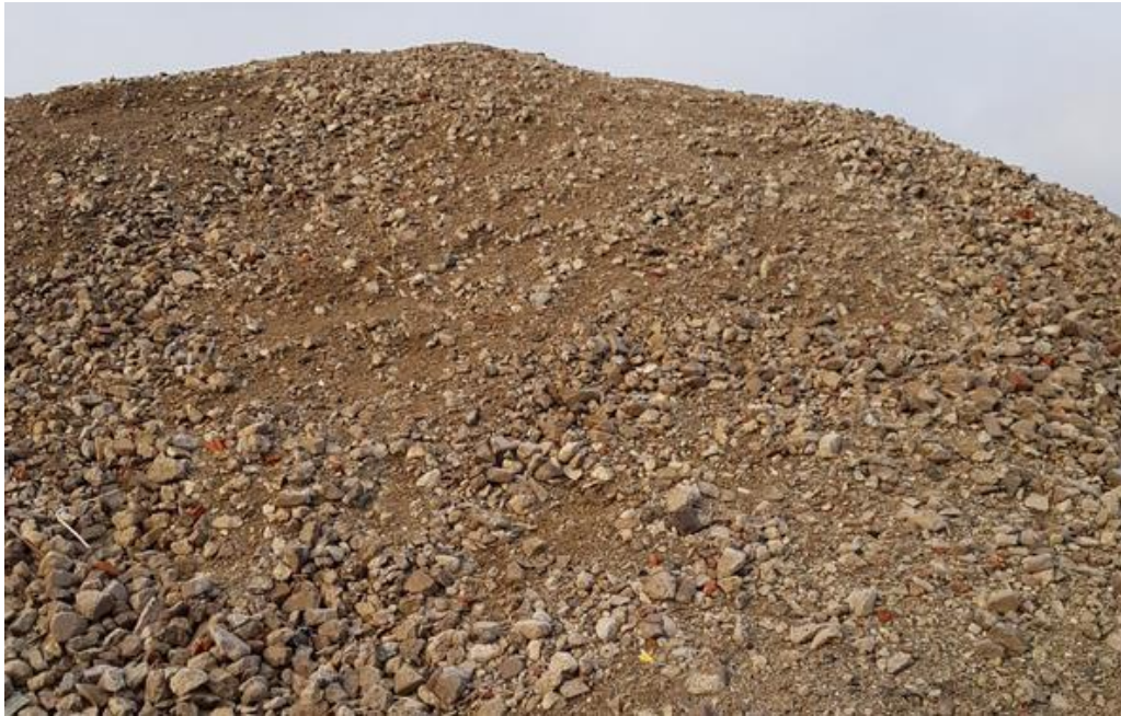
Figure 8. MARA-approved recycled aggregate from demolished concrete with particle sizes 0-150 mm.
