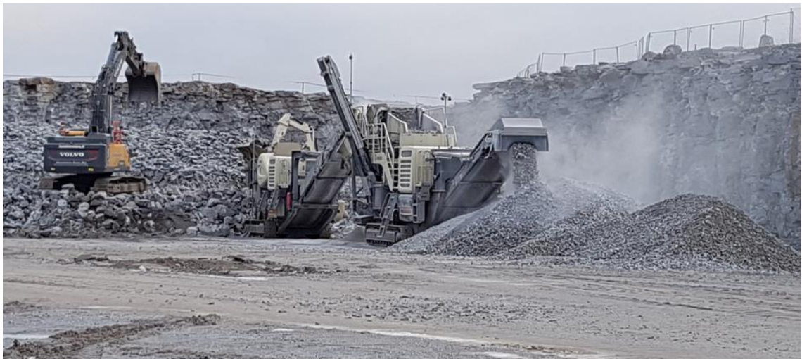
Figure 7. Crushing equipment used in small-scale production of natural aggregate in southern Finland.
