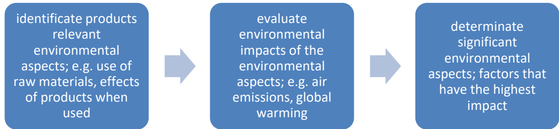
Figure 5. The steps to recognize relevant environmental aspects (adapted from [1])
