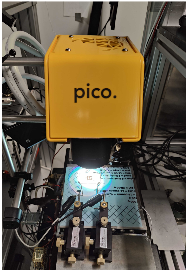
Figure 2.7. The illumination head of the G2V Pico solar simulator.
