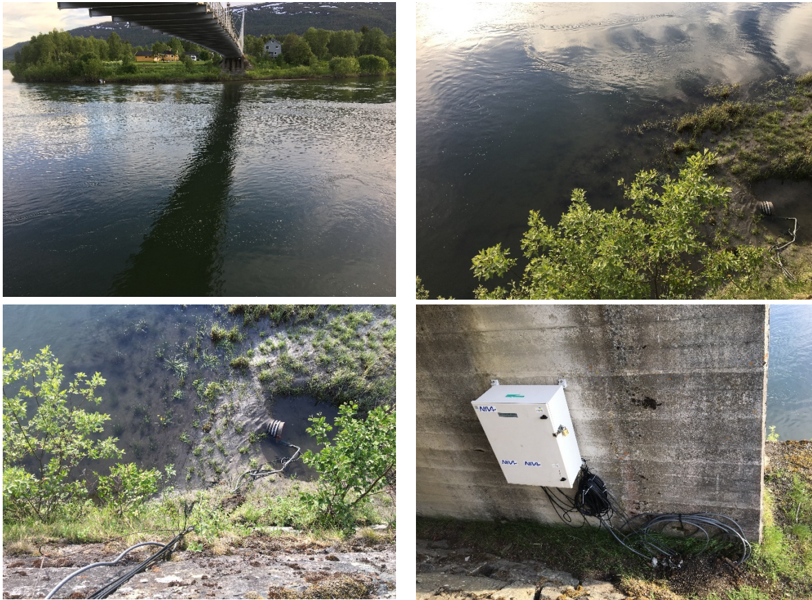
Figure A2. Photos from the Måselva sensor station showing the location of the sensor (near the old E6 bridge at Moen), location of the pipe through which sensors are deployed and the logger box.
