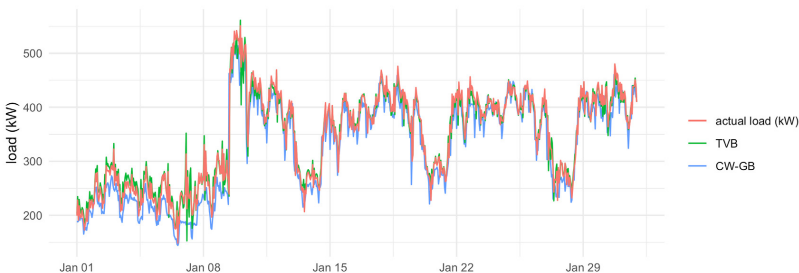
Figure 1. Actual loads (kW) for January 2018, and the predicted loads from TVB and CW-GB models, both models with the dependent variable lagged 1 hour.
