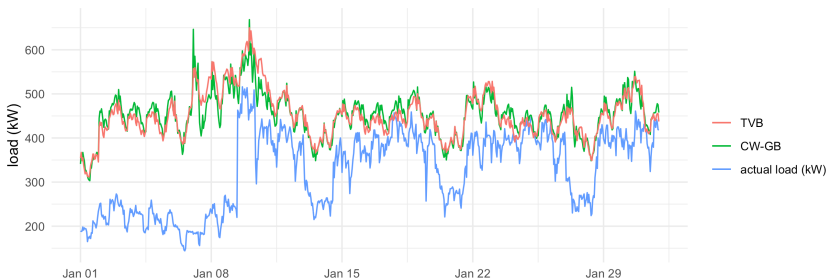
Figure 2. Actual loads (kW) for January 2018, and the predicted loads from TVB and CW-GB models, both models without the dependent variable lagged 1 hour.
