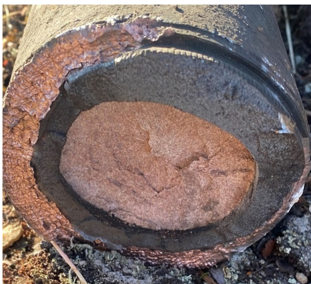
Fig. 2. German 10.5-cm HE projectile cut with flexible linear-shaped charge.
