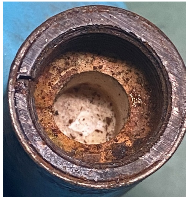
Fig. 3. German 20-mm HE projectile mechanically disassembled.
