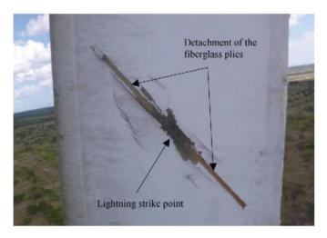
Figure 2. Damage from lightning to a turbine blade [10]
