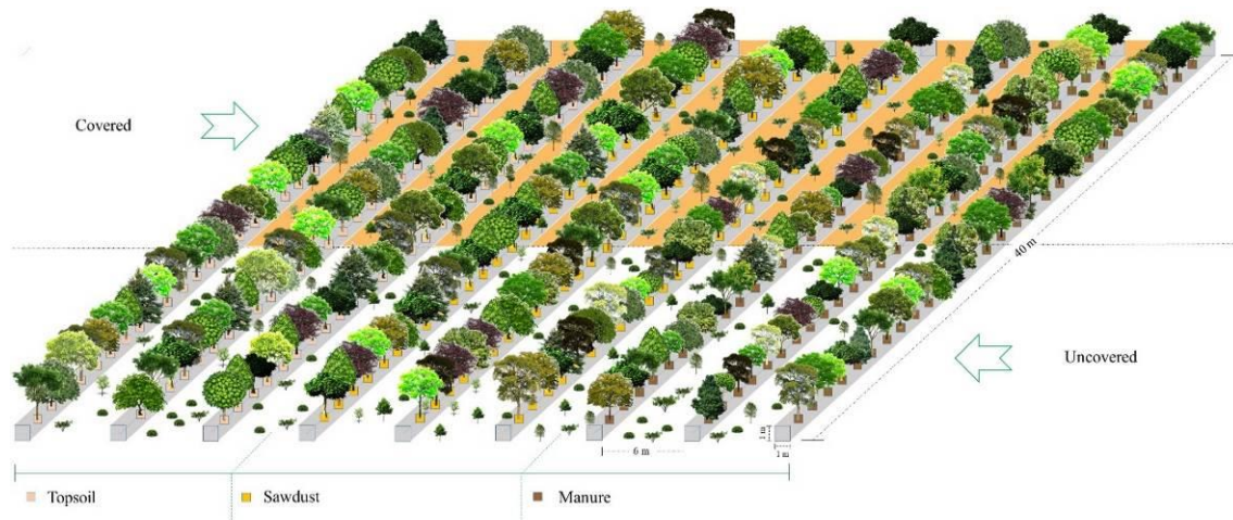
Fig. 2. Simulation of the experimental area with 18 months of implementation and the distribution of topsoil, sawdust and manure treatments, where 50% of the area was covered with sawdust in forest restoration areas after kaolin mining, PPSA mine, Eastern Amazon, Brazil
