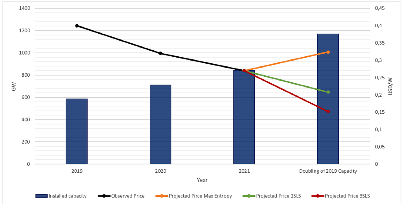
Fig. 3. Solar PV prices, installed capacity, and projections by using the estimated learning rate with different econometric methods (Notes: Data taken from [52]. Prices presented in second axis.).
