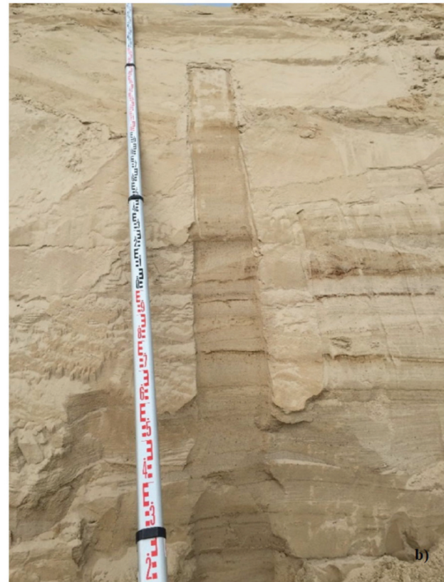
Fig. 5. Micro-layering over approximately 4 m depth as observed during excavation works.
