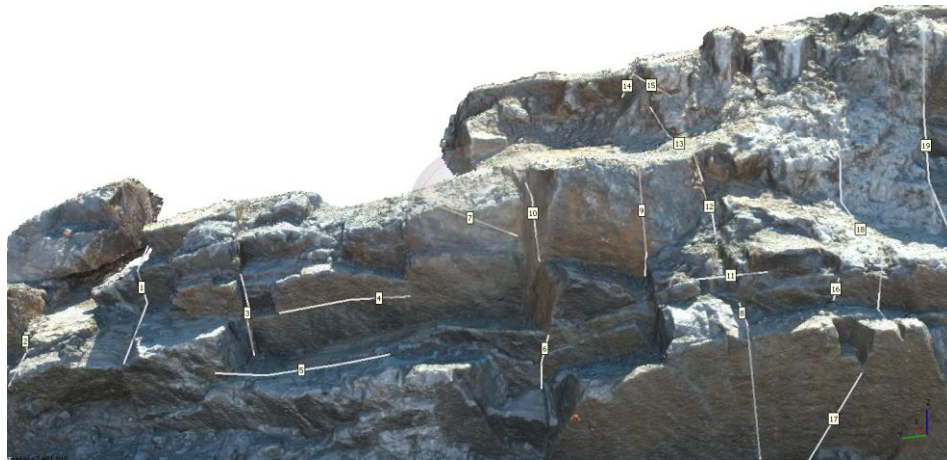
Figure 3. Annotation of rock joint traces using polylines in a dense point cloud. An example from a rock cut from Dataset 1.
