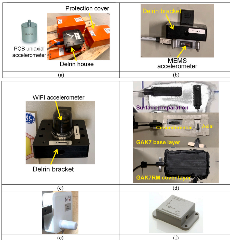
Fig. 3. (a) Retrofitted biaxial accelerometer using two PCB uniaxial accelerometers; (b) MEMS triaxial accelerometer mounted on Delrin bracket with magnet fixture; (c) Wireless accelerometer mounted on Delrin bracket; (d) Installation process of SGs; (e) Gateway transceiver for wireless accelerometers; (f) Biaxial inclinometer.
