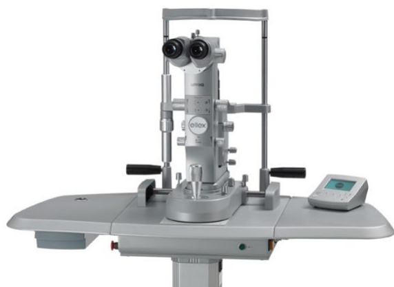
Figure 2. An example of a YAG laser used to perform LPI. 5
