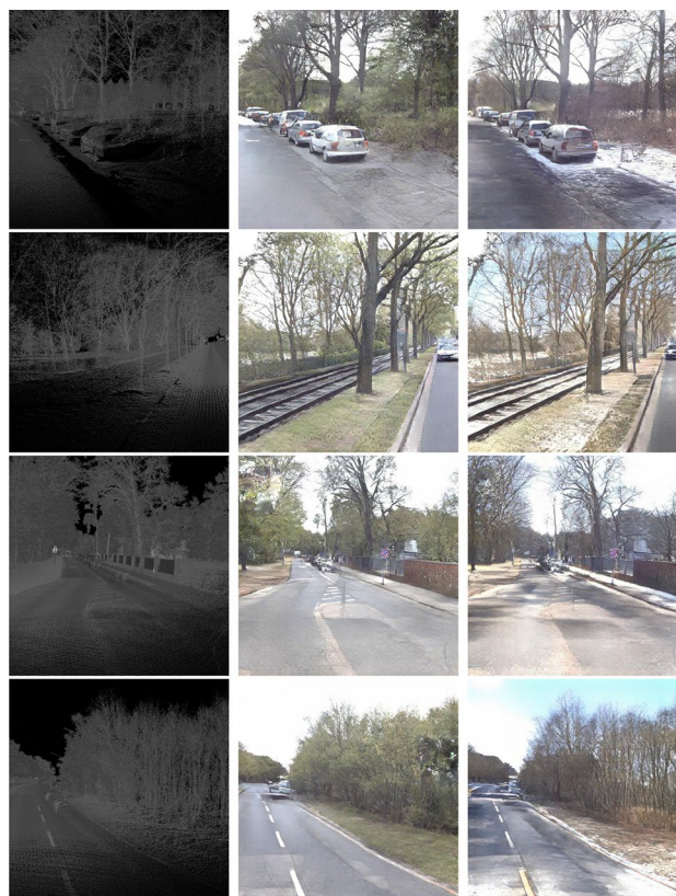
Fig. 6 Examples for summer (middle) and winter (right) representation of the same input point cloud coloured by reflectance (left) in Hannover (row 1 and 2) and Karlsruhe (row 3 and 4)
