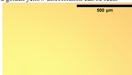
Fig. 4. Optical microscope image of laser annealed TiO 2 -Sol-Gel layer generated with a DC of 18 % and 62 mm/s using an axis system
