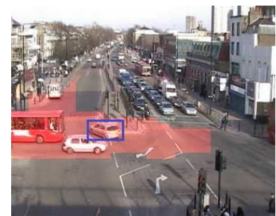
Figure 3: Examples of detected anomaly caused by emergency vehicles using our GP models (abnormal regions are denoted in red whilst the corresponding abnormal object is highlighted with a box).
