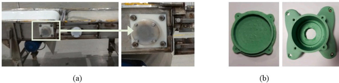
Fig. 1. Example of spare part: square bearing housing; (a) Commercial part assembled in a conveyor belt in a fishery's factory; (b) Recycled part made from plastic waste by 3D printing technology.
