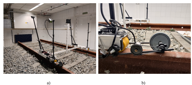
Fig. 1. Inspection system prototype. a) Inspection trolley. b) Displacement measurement system.
