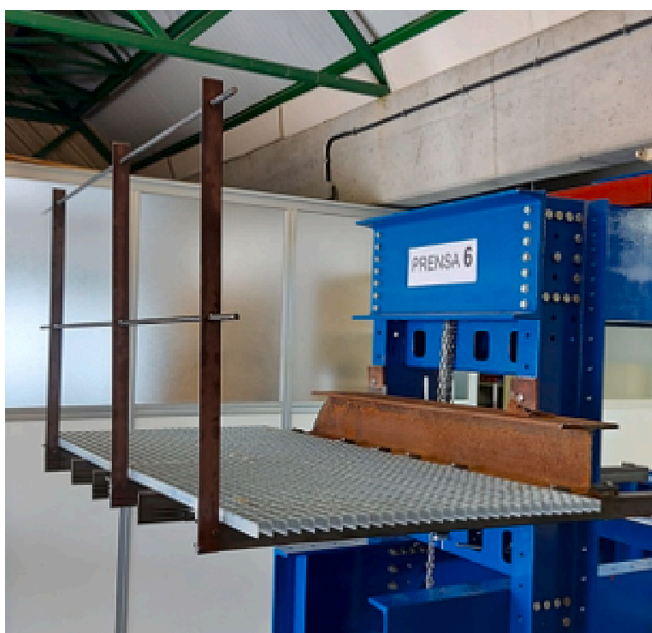
Fig. 9. 2-meter section of the platform system assembled in the laboratory.
