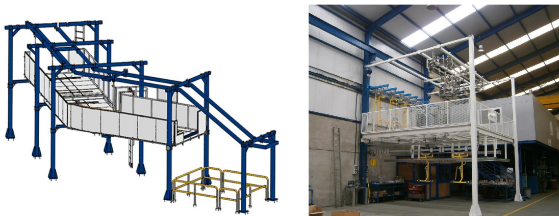
Figure 2. Example of a support structure for industrial conveyors.
