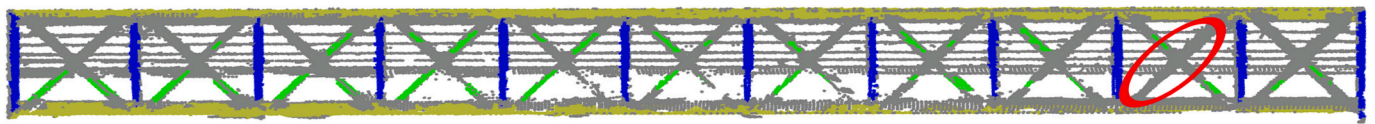
Fig. 39. Vertical face of case study II bridge segmented. The error is marked with a red circle. (For interpretation of the references to colour in this figure legend, the reader is referred to the web version of this article.)
