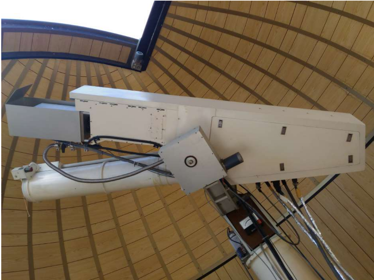
Figure 1. The Rome/PSPT telescope in the host-dome at the INAF Osservatorio Astronomico di Roma in Monte Porzio Catone (Rome, Italy). The telescope has an equatorial mount and body comprising a lower tube that includes the objective lens and its dust cover, and upper part with the secondary optics and appended recording device. The guiding system is located in the back part of the telescope.
