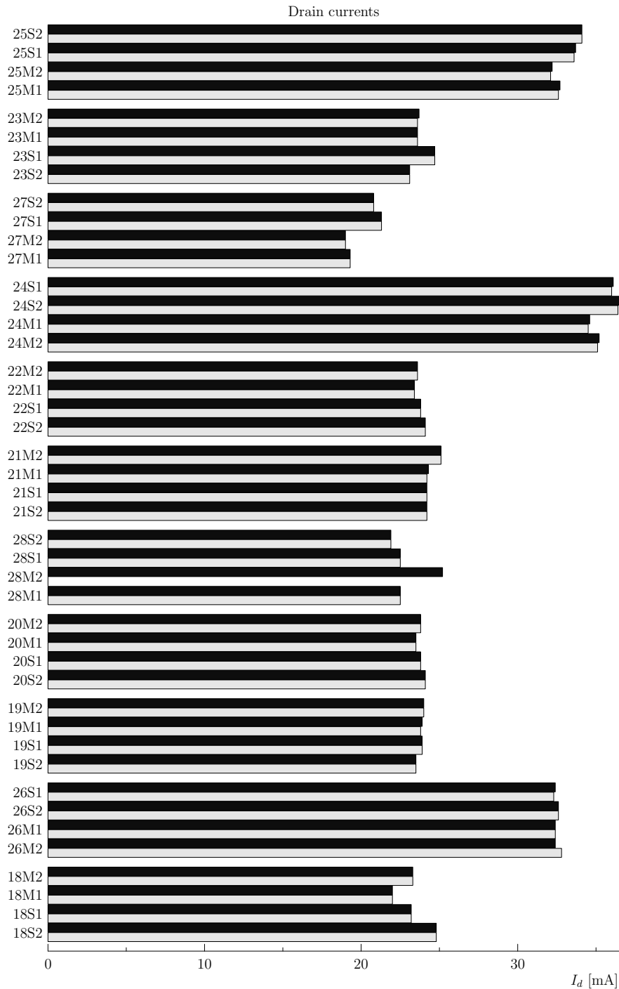
Figure 2: Comparison between the drain currents measured during the pre-cooling WFT (light bars) and the post-cooling WFT (dark bars). Data for #28 M2 was lost due to a TMH failure.
