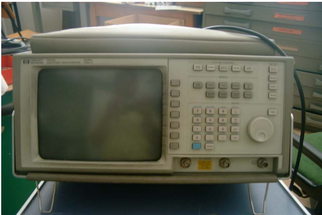
Fig. 5 HP Digital Oscilloscope front view
