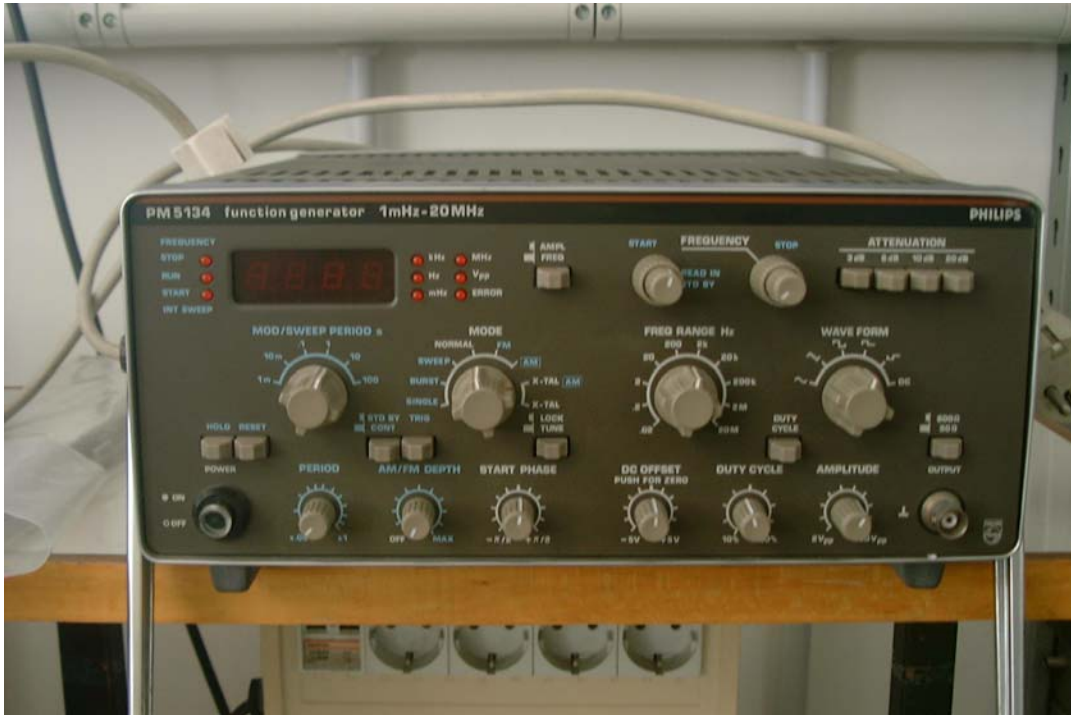
Fig. 4 Philips PM5134 function generator front view
