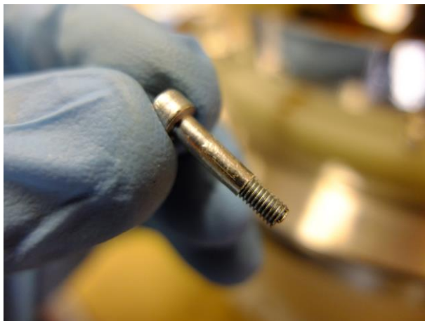
Figure 23. Left: Modified screw to permit the mounting of the cartridge body. The screw has been surrounded by well matched aluminium tape. Right: GARD proposal for alignment pin to be mounted on the M3 thread.
