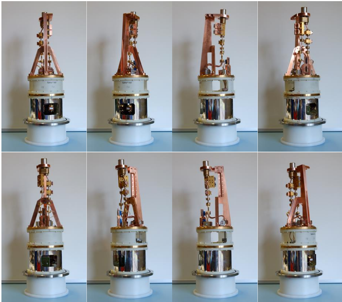
Figure 29. The Band 2+3 (67-116 GHz) Variant 3 as integrated and ready to be inserted into the ESO NAOJ cryostat for cryogenic tests.
