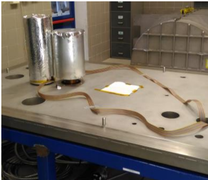
Figure 2 The dry run setup only consists of the two coolers in the chamber. Their cold stages are protected by radiative shields visible in the figure. The left (and higher) shield covers the 4K cooler while the shorter right shield surrounds the 20K cooler cold stage. The harness inside the chamber is used for reading temperature sensors, located in
