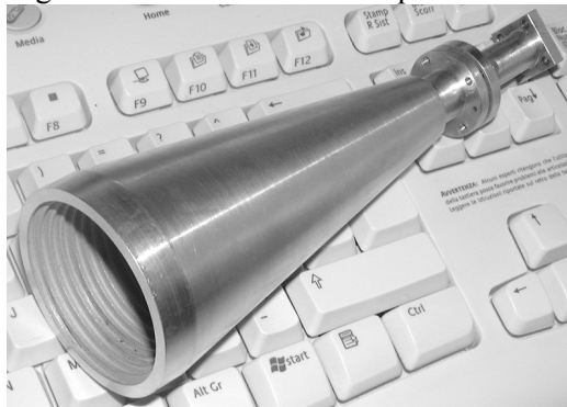
Figure 4 Sky horn. This horn is the LFI EBB horn connected to the circular / rectangular waveguide transition.
