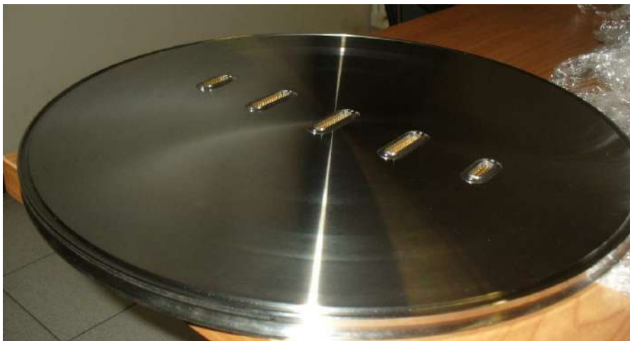
Figure 6-18: PANTER flange with dedicated connectors
