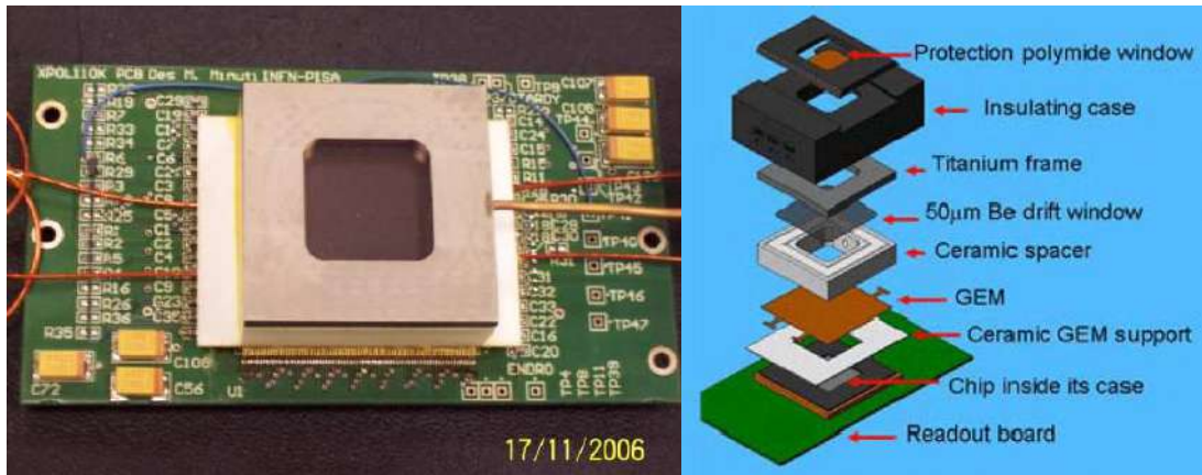
Figure 5-5: The LEP Detector-FEE Assembly
