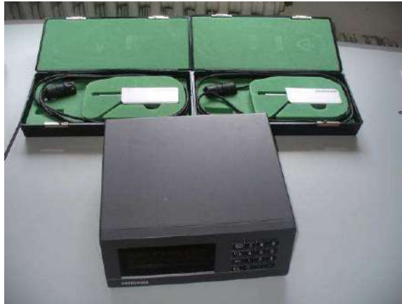
Figure 6-17: Heidenhein sensor for the rotation calibration
