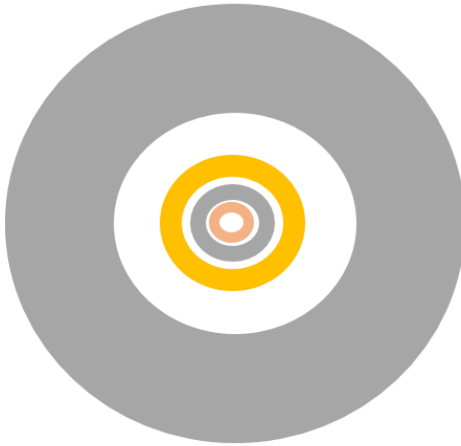
Figure 6: A possible multilayered shielding consisting of 4 cm Al (grey) + 2 mm Au (yellow) + 1 mm Al (grey) + 1 mm Be (pink). In this configuration the background induced from diffuse X-ray photons is suppressed (thanks to Au), while the background induced by cosmic protons (green curve) is about the same as in the case of a 4 cm Al shell only (blue curve). However, in this configuration a flux of spallation neutrons \sim 3 times larger is found. The units in the plot are arbitrary as the both the background curves refer to the same closed spherical shell test geometry
