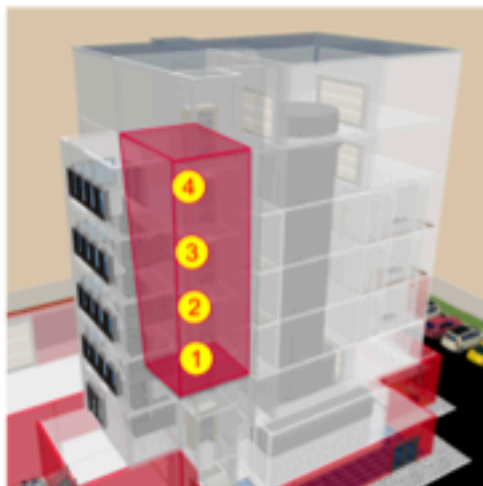
Figure 1-39. Building volume dedicated to the technical rooms.
