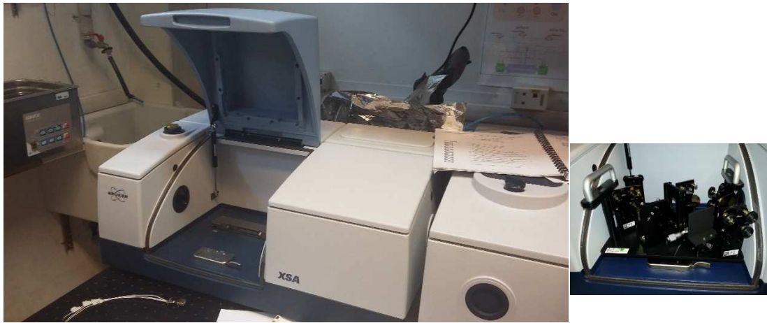
Figure 2: Fourier Transform InfraRed (FT-IR) spectrometer used to characterize the dichroic filter (on the left); optical setup used to record the transmittance with parallel beams (on the right).
