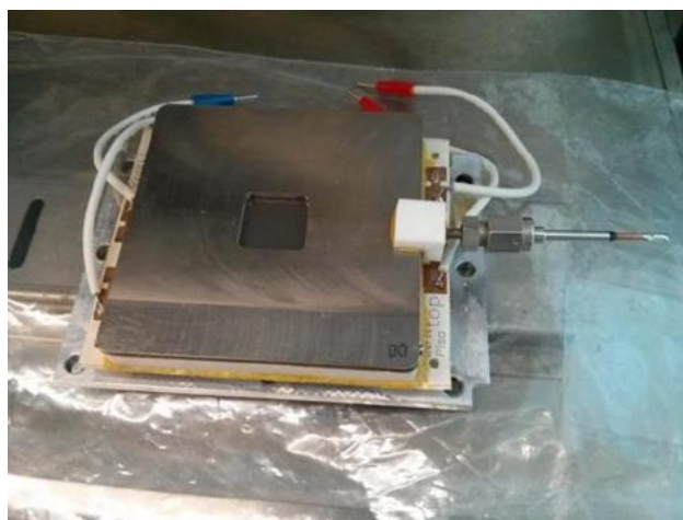
Figure 18 Picture of the GPD serial number 14, the Be window is protected by a plastic cover (to be removed during test), the gas tube and its connector is clearly visible.
