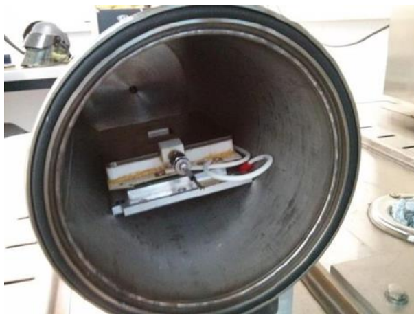
Figure 19 Picture of the GPD serial number 14 installed into the vacuum chamber (at OIA).
