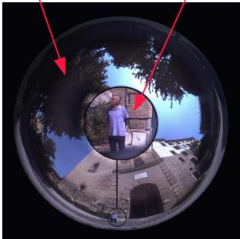
Fig. 1. (top) The BPL optical diagram, (bottom) example of a frame/snapshot as it appears RAW in the imaging device.
