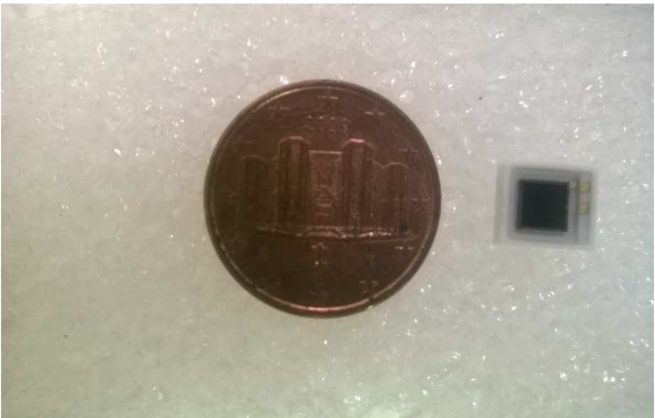
Figure 2: Picture of the SiPM by Hamamatsu, compared to a 1 cent EUR coin
