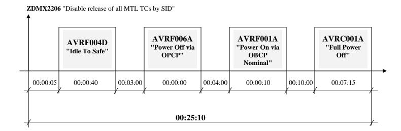
The block "AVRF004D" has been added to force the instrument in the SAFE state, in case for some unknown reason, VIRTIS is in the IDLE state, where the subsequent blocks would be rejected
