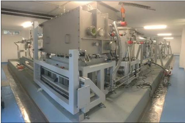
Fig. 1. BEaTriX facility realized at the INAF-OAB laboratory. The vacuum chamber holding the optical components is visible in the foreground. Beam generation and handling occurs in the “short arm” on the left side. The 12 m tube (the “long arm”) for X-ray propagation to the focal plane is on the right.
