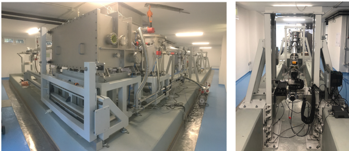
Figure 1. BEaTriX: view of the laboratory from the vacuum chamber containing the optical elements (left), and from the detector flanged at the end of the 12 m vacuum tube (right)
